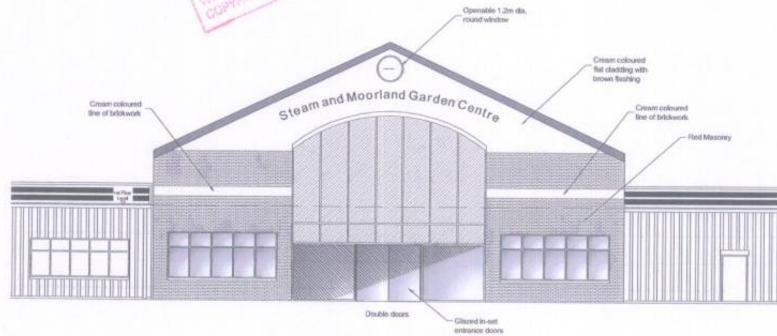
Proposed Front Elevation Scale 1:100
